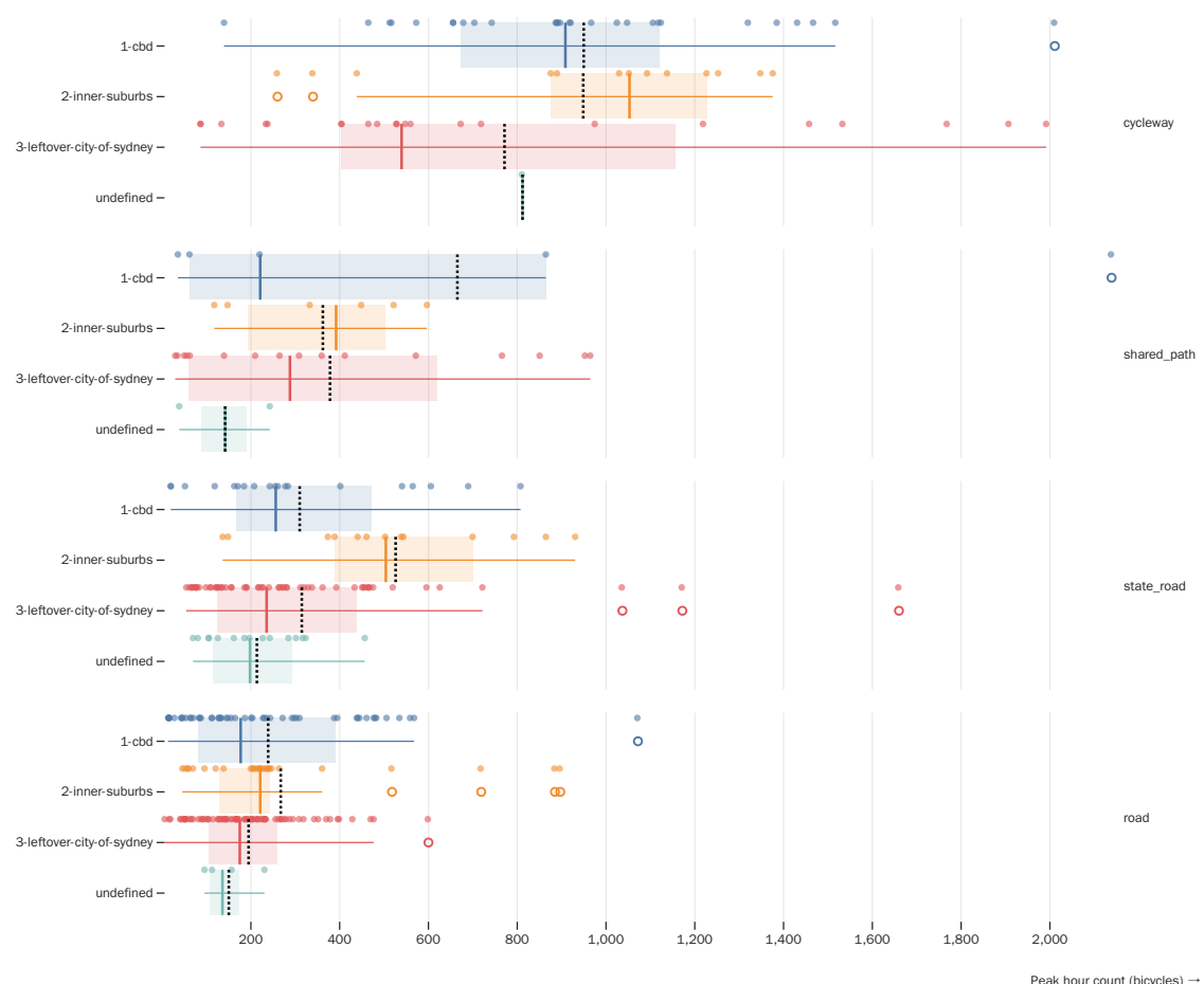
Figure 31: Peak hour volumes of virtual screenlines and new automatic counters - by area, faceted by infrastructure type. Dots are individual sites. Box is IQR, dashed line is average, solid is median, whiskers show 1.5x IQR.
